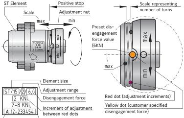
After loosening (approx. 1 rotation) the locking screws  $(E_3)$ , the adjustment nut can be turned to adjust the disengagement setting. Incremental values are marked on the adjustment scale. After adjustment, the torque setting is secured by tightening the locking screws  $(E_3)$ .
