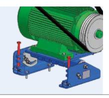
adjust with M20×1.5 screw (for tightening = screw block downwards)
