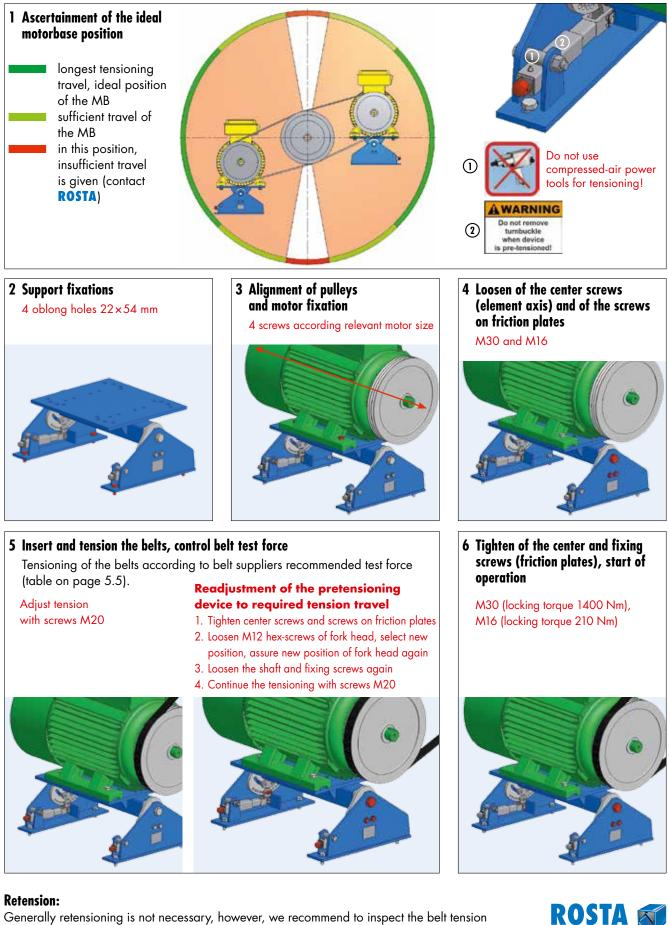
Generally retensioning is not necessary, however, we recommend to inspect the belt tension after a few days of operation (after "running-in" of the belts).
