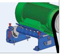
4 Loosen of the shaft screw (element axis) and of the screws on friction plate(s) M20 and M16
