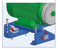
6 Tighten of the shaft and fixing screws on friction plate(s), start of operation
